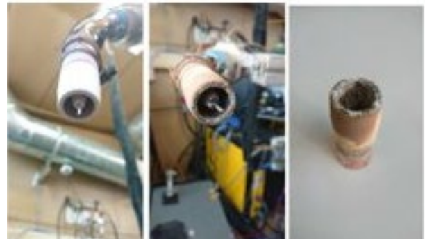
Left to Right: Applied to nozzle; Nozzle view after welding; nozzle removed from gun and minimum spatter.
